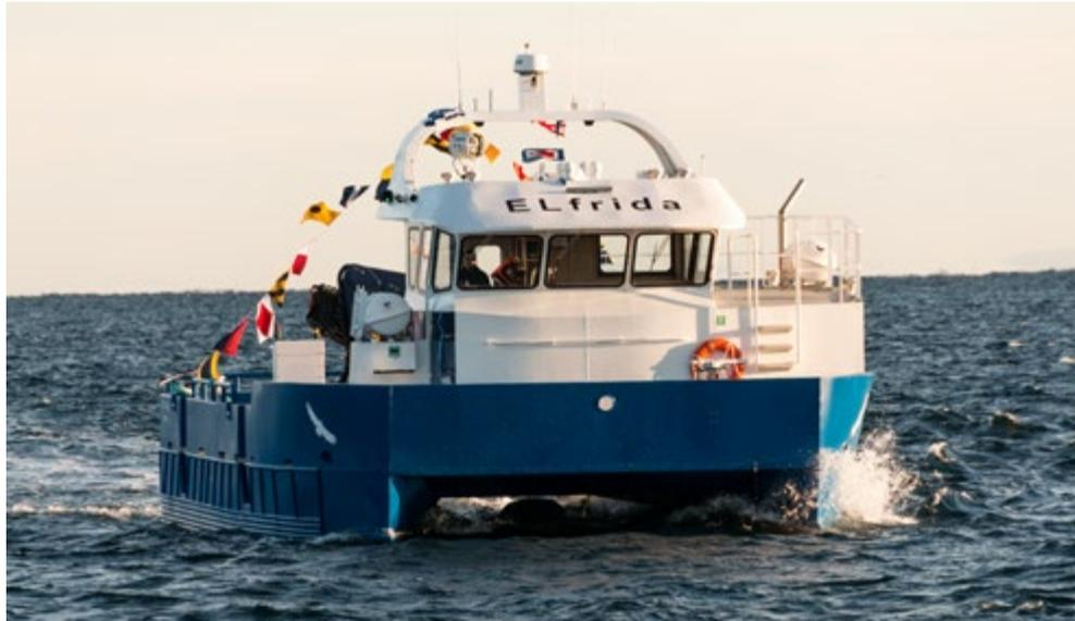
Since 2017, Salmar Farming has been using the hybrid-electric workboat *Elfrida*, which runs on electricity 80–90 % of the time. Photo: Enova
