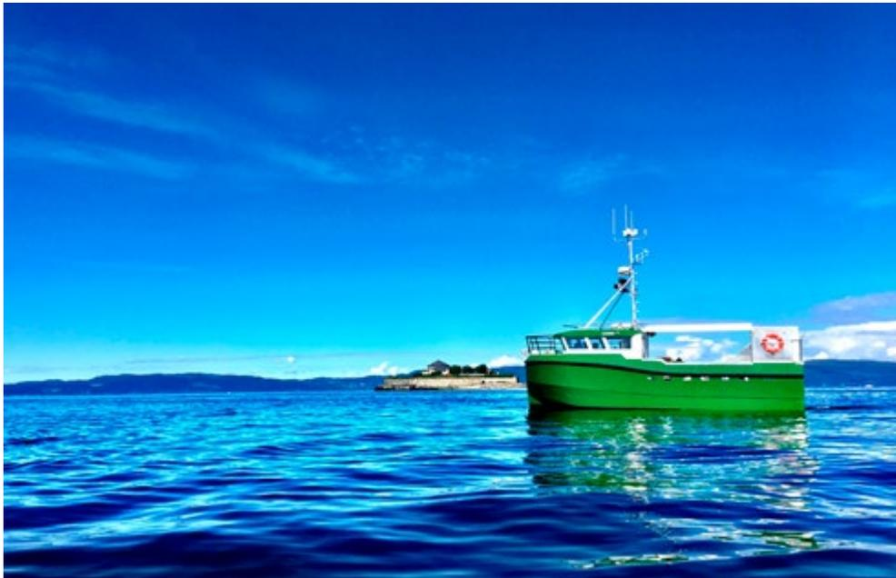
**Karoline is the world's first hybrid fishing boat with an electric propulsion system. The vessel is 11 metres long, and has a diesel engine for use to and from the fishing grounds. The battery packs provide the vessel with enough power for two hours fishing and 45 minutes of propulsion.**
